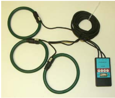
Three FCA-Flex sensors with Amplifier.
