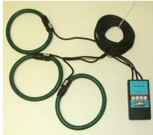
THREE SENSORS WITH AMPLIFIER Triple-probes are hard-wired to the amplifier
